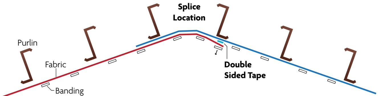
In some instances, where a building is too wide for the Energy Saver FP™ fabric to be installed from eave to eave in one full piece, field splicing may be required. On a double slope building, this will be done at the first purlin down from the ridge. On a single slope building, the splice will be made at a pre-determined purlin mid-slope. Follow the detail above to do this.
