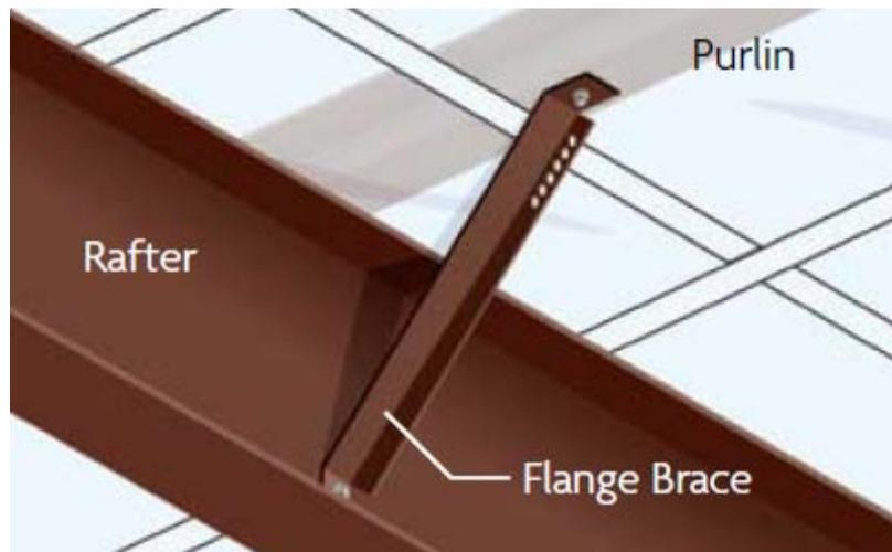
***Anyone who implies that you can or should relocate flange braces is potentially putting your company at risk. Alternate connection is possible but should not be considered without approval from the steel building manufacturer prior to ordering the building.***
